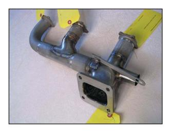
We stock a complete set of overhauled exhaust parts for the TSIO-520 or TSIO-550 powered Malibu.
