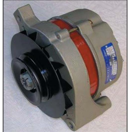
Malibu Power & Propeller stocks both gear-driven and belt-driven alternators for the PA46-310P Malibu. All alternators are rebuilt by Aerotech and have excellent service life. One alternator won't sustain flight in night-time or icy conditions. We recommend replacement of each alternator every 500 hours to reduce the chance of in-flight failure. With Malibu Power & Propeller's low prices, overhauled alternators are inexpensive insurance, giving you peace of mind every time you fly.
